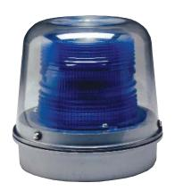
The Model 531A Strobe features an incandescent constant-on lamp for locating the emergency telephone, and a high-intensity Xenon tube for flashing operation when the telephone is in use. In addition, the strobe provides a secondary contact output for activation of external auxiliary equipment.
